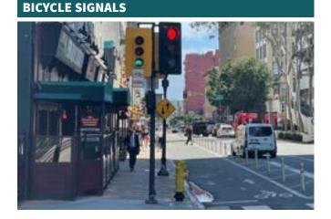
**Bicycle signals** create a signal phase at intersections that is specifically for bicyclists and does not conflict with vehicle movements. A bike signal must be installed on the far-side of an intersection with red, yellow, and green indicators in a bicycle shape, while a near-side signal is optional to improve visibility.
