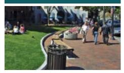
**Curb extensions**, also known as bulb outs, extend the curb line into a roadway at a crossing location. Curb extensions can increase the area available for pedestrians to safely wait before crossing an intersection, reduce crossing distance, and increase pedestrian visibility. Curb extensions can be semi-permanent (striping and delineators) or permanent (sidewalk with curb and gutter), depending upon the characteristics of the roadway.
