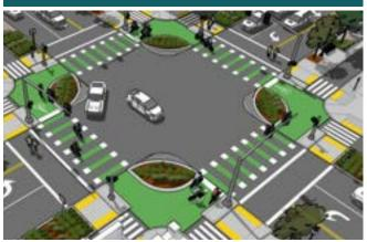
A **protected intersection** physically separates bicyclists and pedestrians from vehicle traffic at an intersection to reduce areas of conflict with vehicles. Protected intersections have separated crossing facilities to reduce crossing distance, enhance pedestrian and bicyclist visibility to vehicles, and encourage lower speeds.
